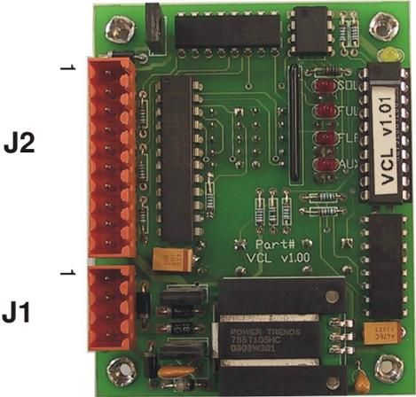
All connections to the board are through the two connectors.
