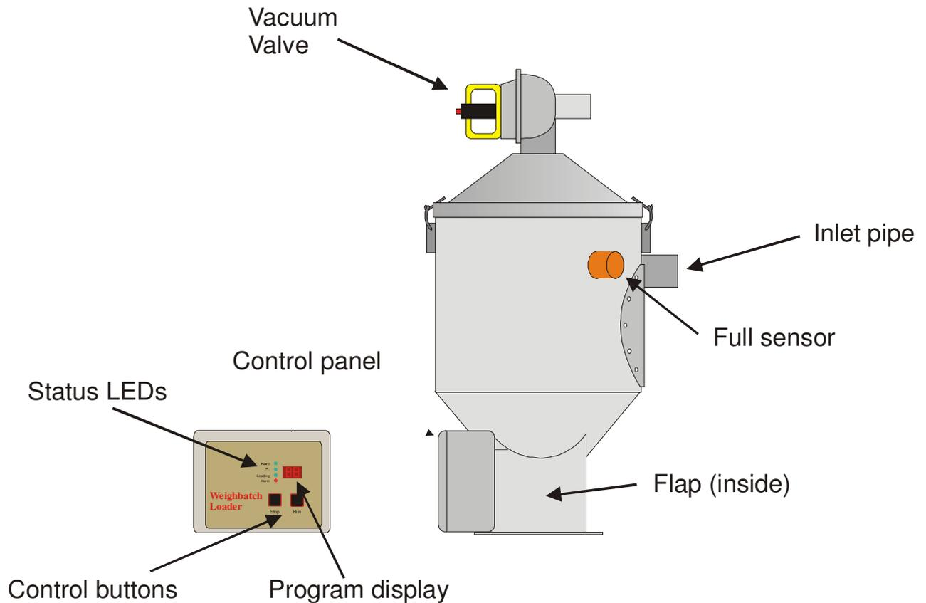
When the Vacuum Valve is turned on, air is drawn through the Loader. The Loader sucks material into the body of the Loader.
