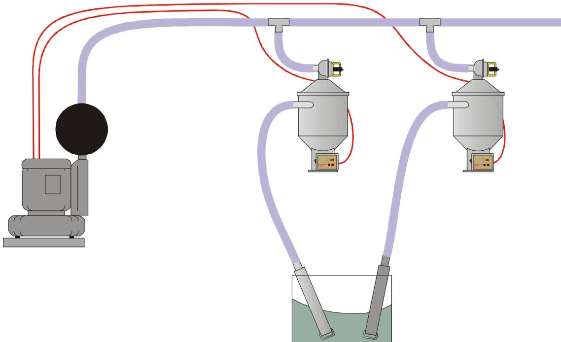
A common vacuum line runs from the Vacuum Pump Filter past each Loader. A "T" junction (or similar) connects each Loader's vacuum valve to this common line using flexible hose. The other hose feeds material from a storage bin to the Loader. A filter just upstream of the Vacuum Pump prevents material and dust from passing through the Pump.
